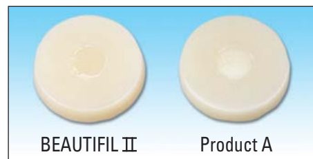
Core before curing and outer ring after curing
